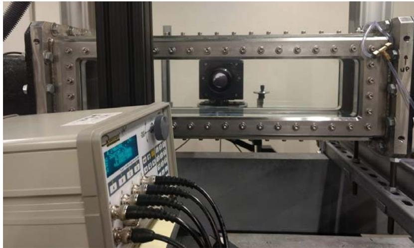
Figure 1: San Diego State University water tunnel test section.
